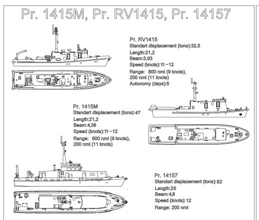
The set includes 3 generations of diving bots. Project 1415 boat were a large series of cutters that were built for the Soviet navy starting in 1976 and are in use up to this day on the rivers and harbors for Russia Project 1415 M is a modernization, and 14157 is a completely new ship.
